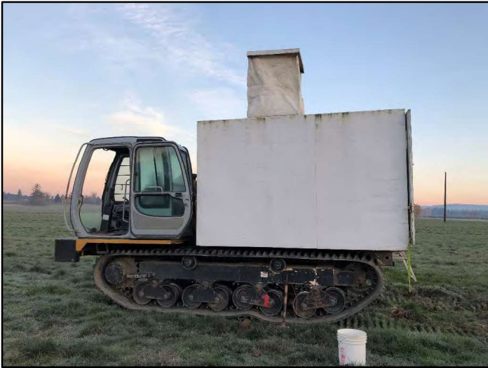
Photograph 1: Conducting CPT-1 sounding with track-mounted cone apparatus.
