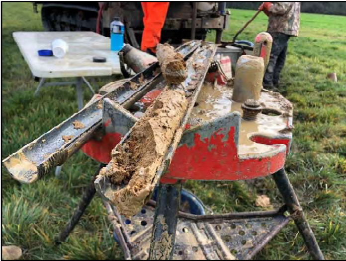
Photograph 9: Split spoon observed from soil boring SB-2 at 40 feet below ground surface.
