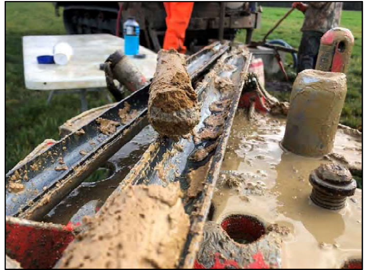
Photograph 10: Gray banding observed in soil boring SB-2 at 40 feet below ground surface.
