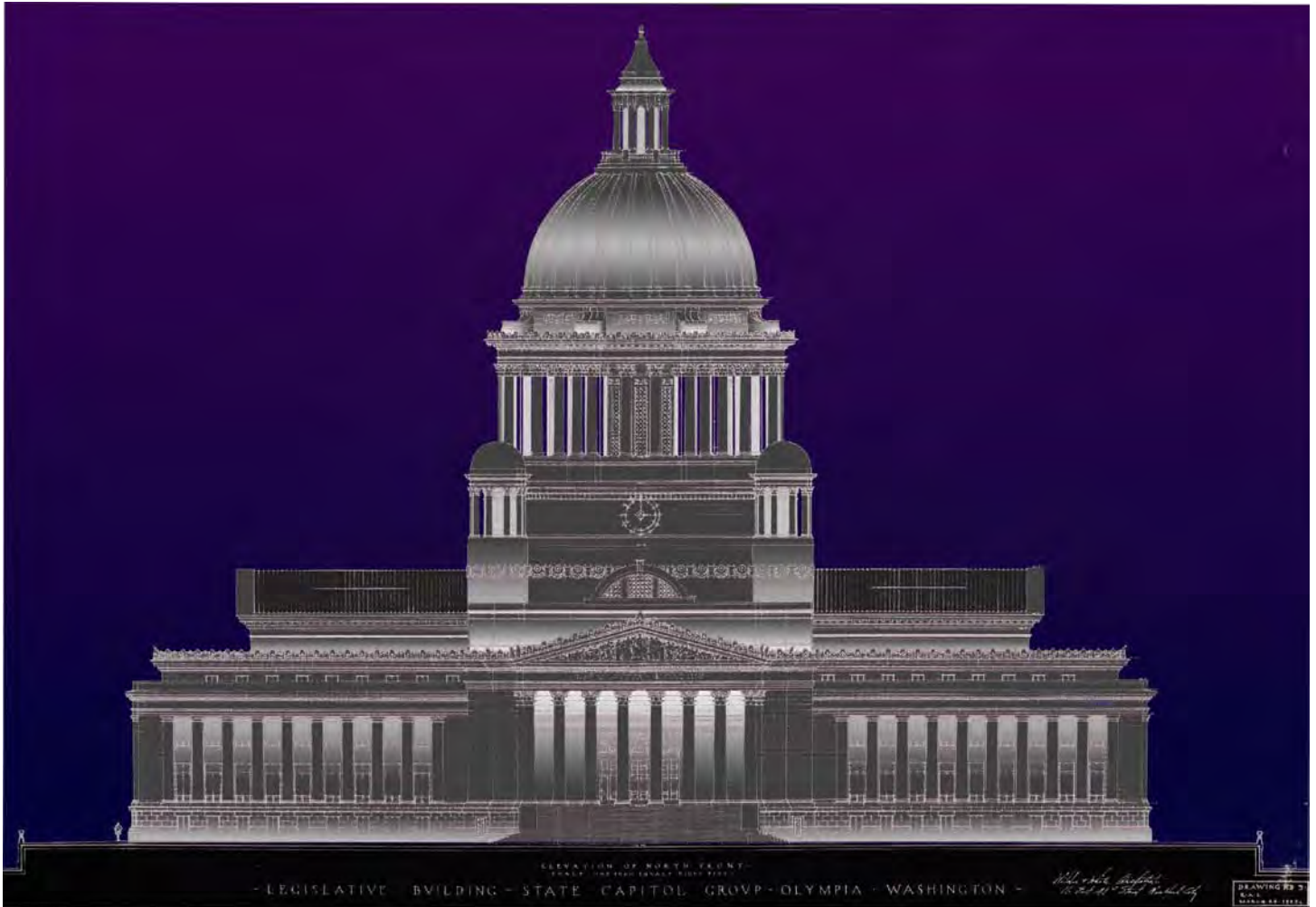
Figure 11.14 One possible alternative for lighting of the Legislative Building. In this alternative, a layered lighting approach is favored over general floodlighting of selected building elements. This layered lighting emphasizes detail, form, and the depth of the architecture. The podium base is uniformly lit to visually ground the building, while lighting within the porticos silhouettes the columns to highlight depth. The entry portico is illuminated to a higher level to aid in wayfinding and provide visual interest. A continuous band of light above reveals the filigree element in silhouette, rendering this element differently at night and providing the viewer with an understanding of the intricacy of these elements. Lighting within the cupolas above and below, along with the columns supporting the dome, provide a different type of layering, as the columns are seen in silhouette toward the viewer, while the inside is illuminated. Finally, the dome itself is softly lit to be seen both within the context of the West Capitol Campus and from distant viewpoints near and far. Together, these elements come together to form a cohesive lighting composition that creates a strong nighttime anchor for the Campus. (source: Dark|Light Consulting, LLC)
