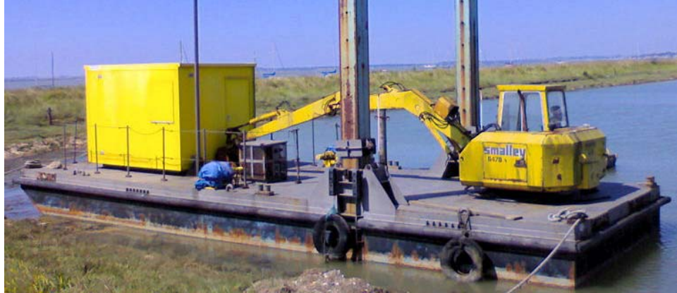
Figure 9. Typical excavator dredge
