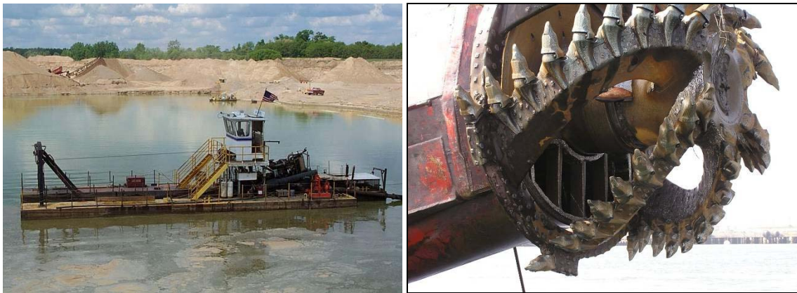
Figure 11. Cutter head dredge (left), close-up of cutter head (right)
