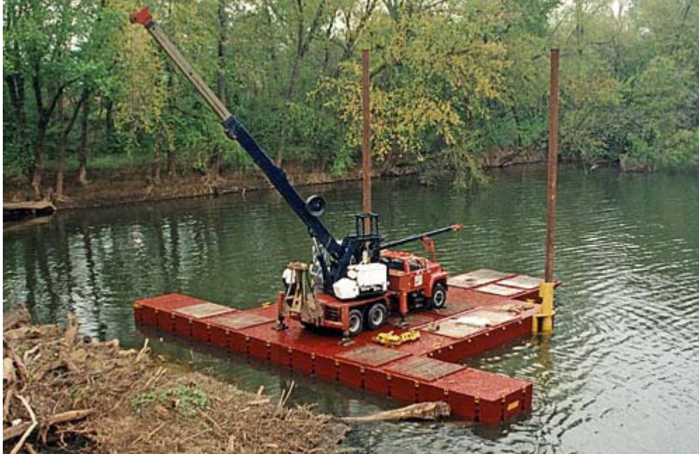
Figure 14. Modular barge system in use (source: www.flexifloat.com )
