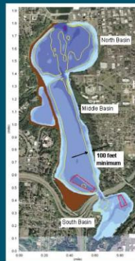
Managed Lake Alternative Existing lake showing proposed dredge footprint (full yellow line) and outline of potential sediment traps (broken red line) Source: Moffatt & Nichol
