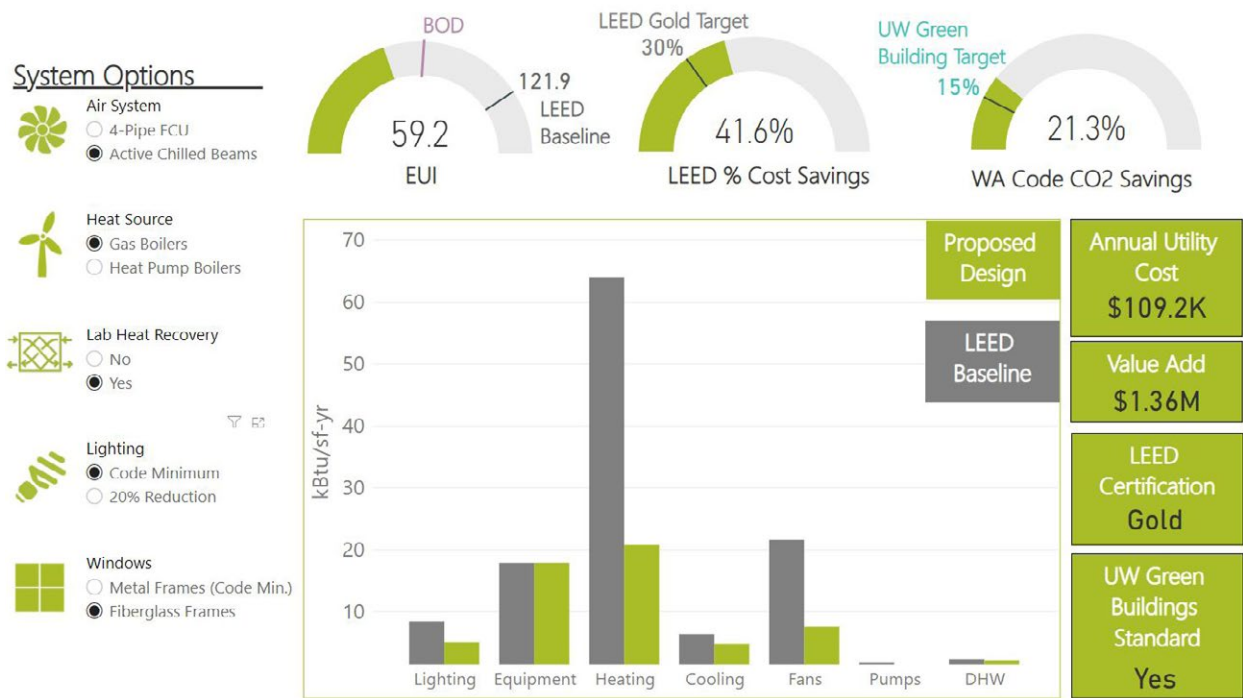
Mithun and our mechanical engineer, Glumac, created this dashboard to help Cascadia College and UW Bothell understand the life cycle cost impacts of alternative energy systems for their STEM 4 project. Changes to the system options on the left are reflected in the data shown on the right.
